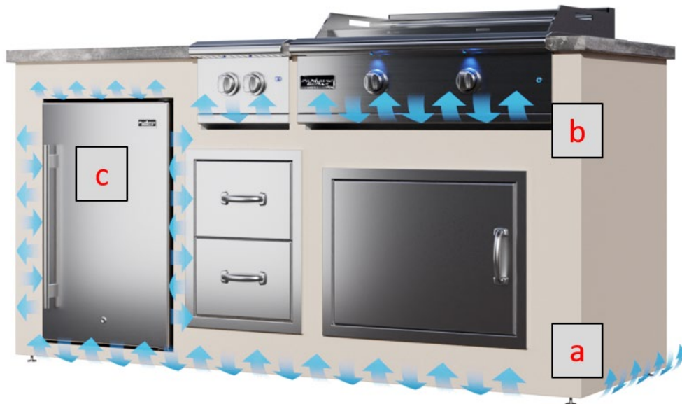
Figure 4 Paradise Grills Island Venting Example
