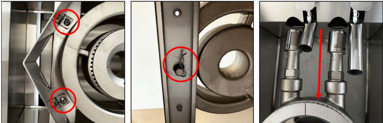
Figure 24 Flame Ring and Burner Removal
