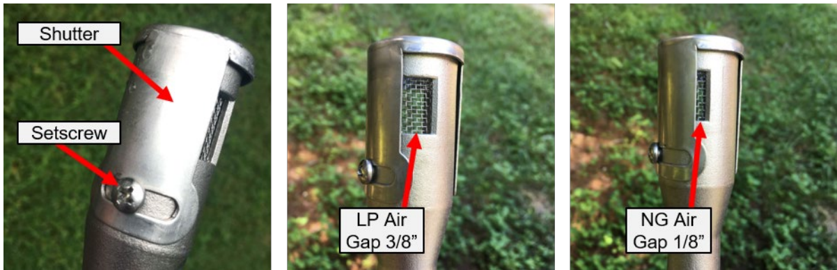
Figure 28 Adjust Air Gap
