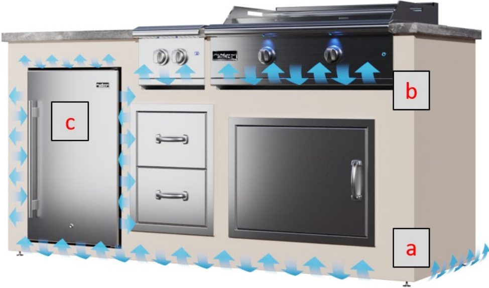
Figure 4 Paradise Grills Island Venting Example
