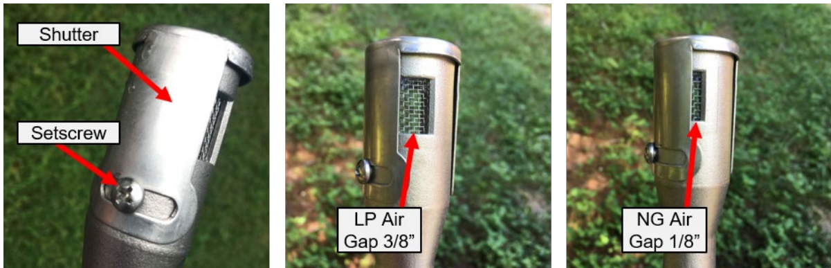
Figure 32 Set Air Gap for Gas Source
