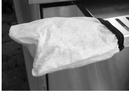
Figure 15 Drip Pan Protective Covers
