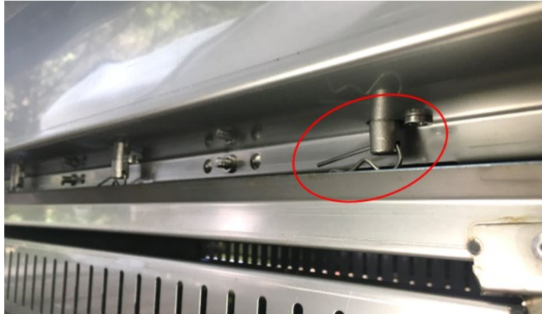
Figure 9 Remove Burner Cotter Pins
