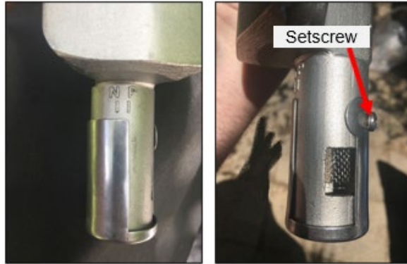
Figure 38 Adjust Air Gap
