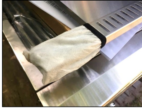
Figure 16 Drip Pan Protective Covers
